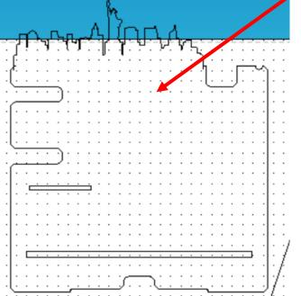
19. Using the *delete part tool* and *delete* the line separating the top and bottom of the clock to join the two parts together as shown.
