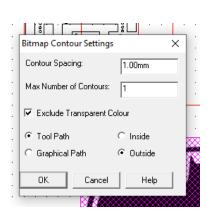
26. A Bitmap contour spacing pop up will appear. This basically traces the image. *Change the contour* from 5.00mm to *0.00mm*.
