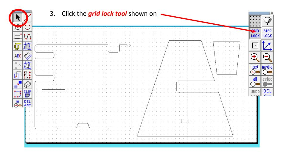
4. You will notice the bed size is bigger. It measures **300mm** x **600mm** the size of the laser cutter bed.
